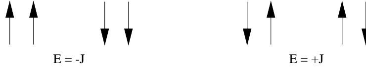
Figure 16.1: The interaction energy between nearest neighbor spins in the absence of an external magnetic field.
