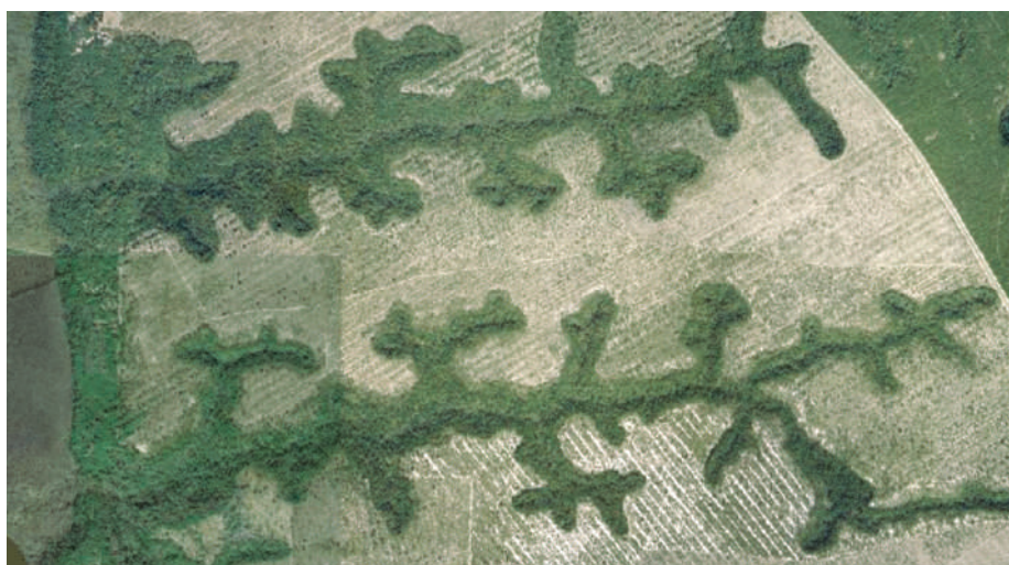
Figure 1 | The Florida channel networks. This aerial photograph shows the well-developed intricately branching channels that are formed by groundwater seepage. Abrams and colleagues 1 show that the seepage rate and the amount of water discharged control the shape and formation of these channels.
